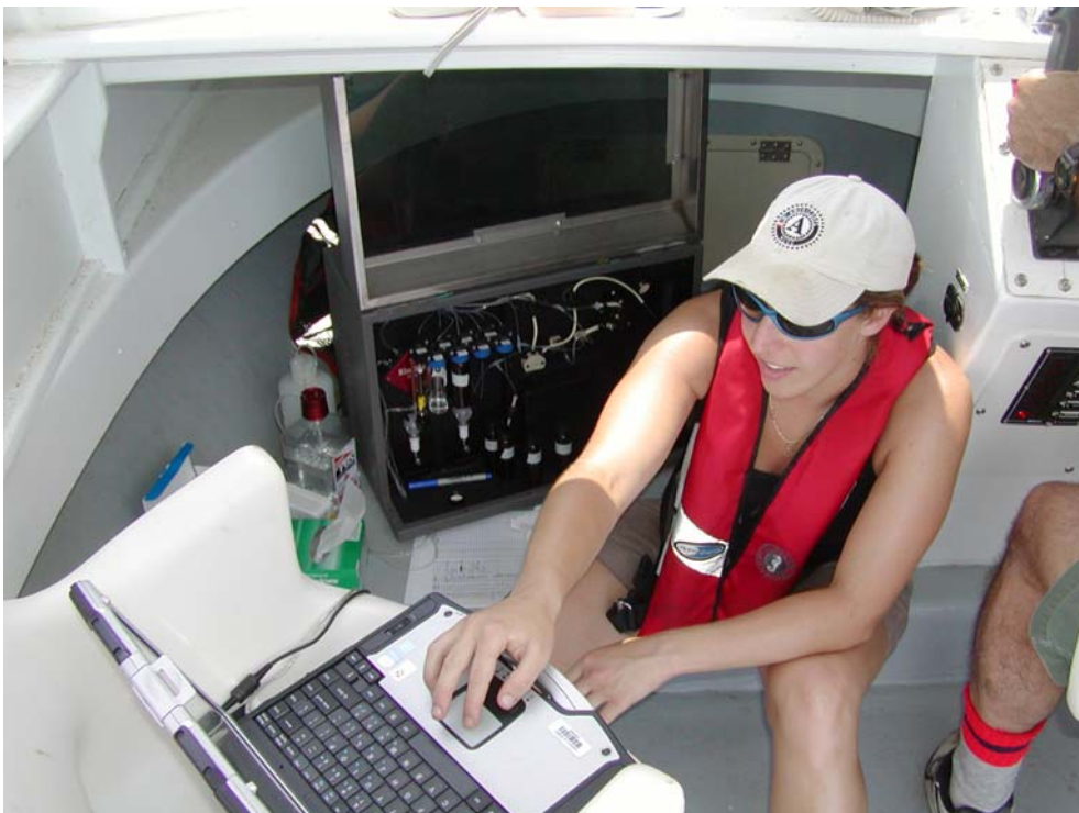
Figure 2. PAH Biosensor on board the VIMS vessel analyzing water samples. Battery power was sufficient to run the biosensor all day. Very high temperatures on board ( >95^{\circ}\text{F} ) caused some baseline stability problems but cooling of the reagents with ice alleviated this problem.
