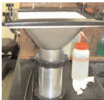
The modified rainwater collector
