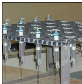
A prototype system being developed to inject air and nitrate into salt marshes contaminated with oil.
