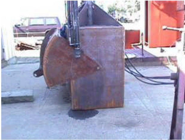
Figure 5-7: Enclosed Excavator with Open Door
