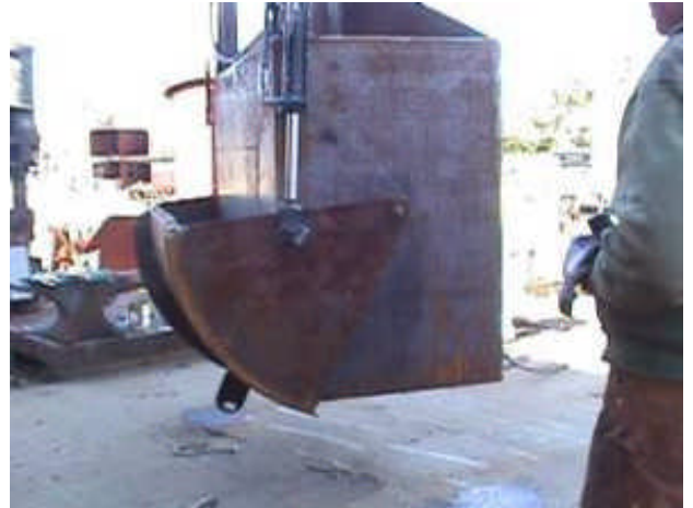
Figure 5-8: Enclosed Excavator with Partially Closed Door
