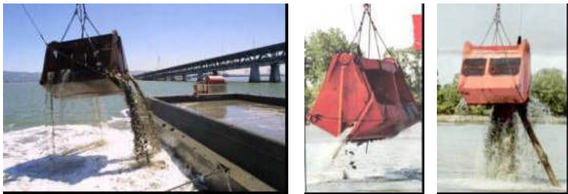
Figure 2-3. Leaky Clamshell Buckets
