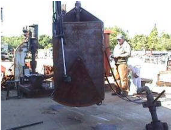
Figure 5-9: Enclosed Excavator with Fully Closed Door
