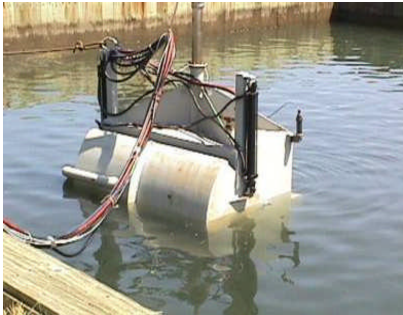
Figure S-3: Pressure-Controlled Excavator Descending Below Surface for Excavation
