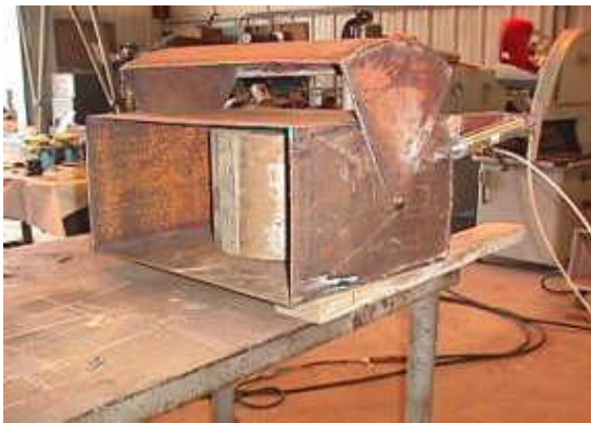
Figure 5-3: Enclosure Door & Hydraulic Control
