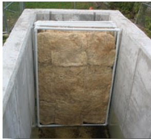
The last straw for polluted runoff? This treatment uses wood straw to remove dissolved contaminants from stormwater.
